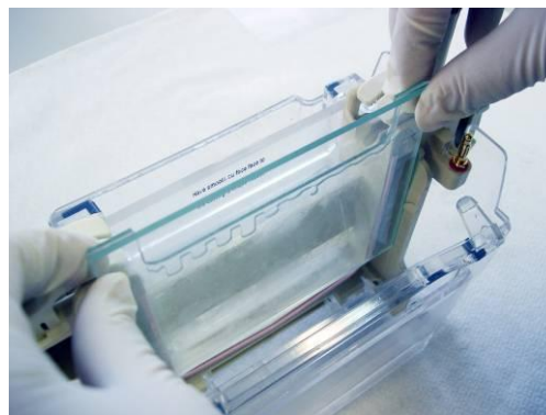
Figure 9. Insert the glass sandwich into the electrode module. Slide the sandwich closely along the pink silicone rubber on the middle part of the module making sure the inside of the gel sandwich risers.
