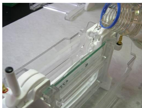
Figure 11. Pour running buffer into the space between the glass plate sandwich and the one-gel gate up until 1 cm from the edge. Make sure the assembly does not leak before pouring running buffer into the surrounding tank.
